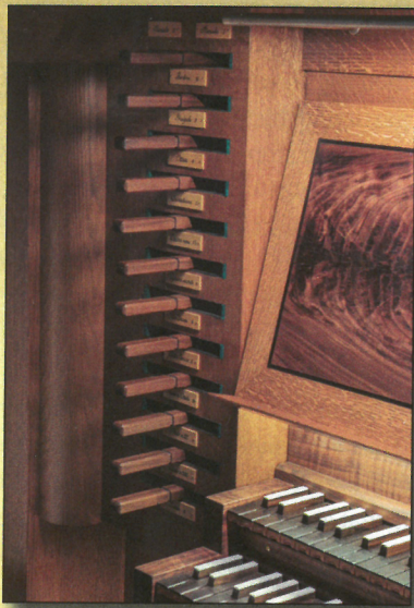
Manual stop levers incorporate a wechschleifen mechanism, enabling stops to be drawn on either manual.
